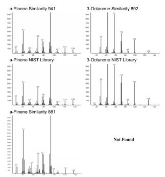
Figure 5. Mass spectra of components 1 and 3 from Figure 4. Upper part represents the data obtained from the GCxGC-TOFMS analysis, second row represents the first match from the NIST library, and the lower part represents the data obtained from the GC-TOFMS analysis.
